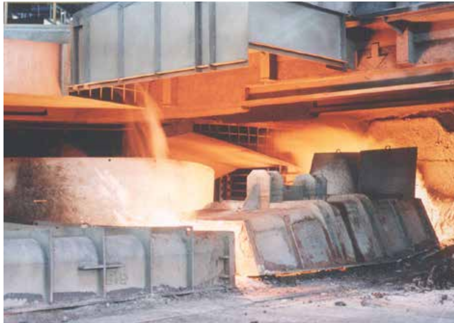
Casthouse taphole extraction
