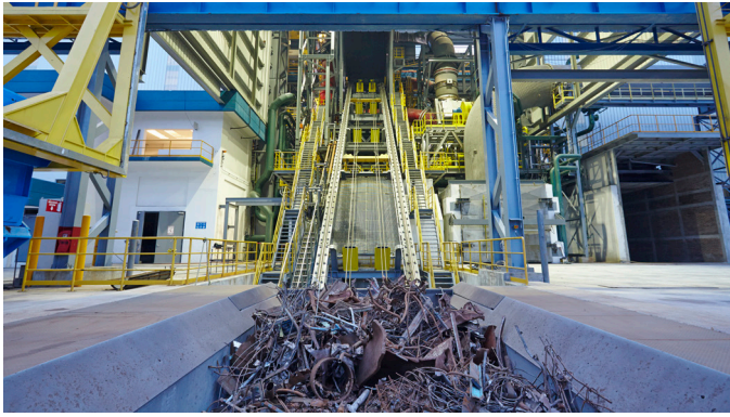
Automated scrap charging system via elevator
