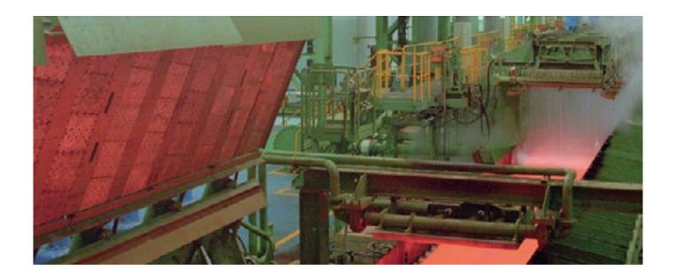
Currently, the most common way to monitor the transformation of iron from austenite to ferrite is by measuring the surface temperature of the steel on the run out table.
